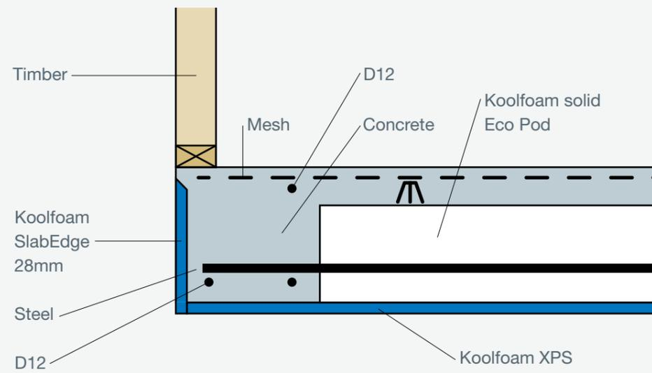
Location and placement of the KoolFoam SlabEdge system to be verified by the architect and or structural engineers. Drawings are representative examples only. Application of Koolfoam SlabEdge to be designed in accordance with H1 Energy Efficiency Acceptable Solutions H1/VM1 H1 VM2 or Verification Methods H1/AS1 H1 AS2.
