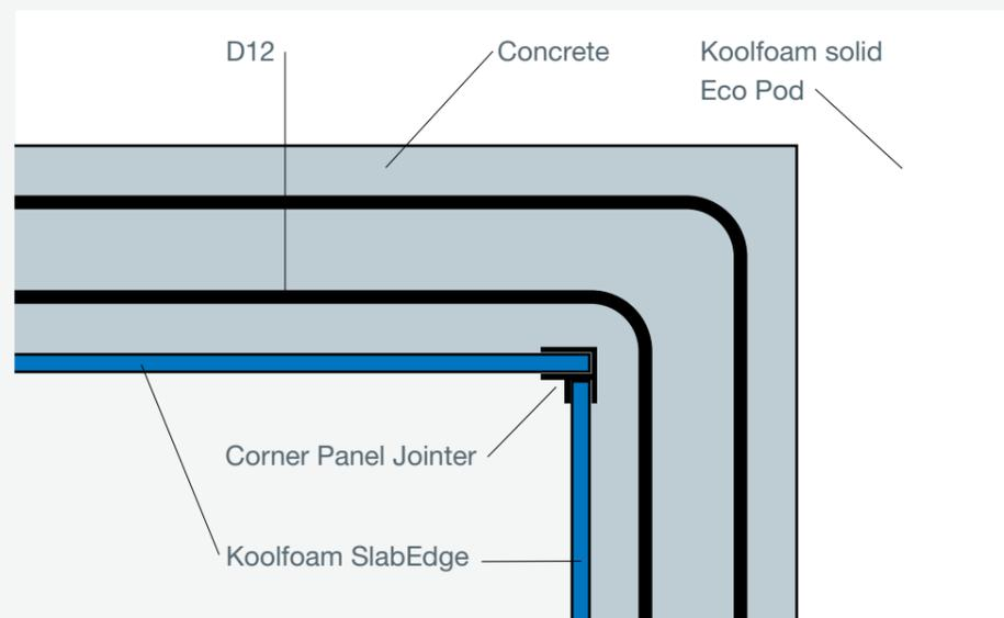
Location and placement of the KoolFoam SlabEdge system to be verified by the architect and or structural engineers. Drawings are representative examples only. Application of Koolfoam SlabEdge to be designed in accordance with H1 Energy Efficiency Acceptable Solutions H1/VM1 H1 VM2 or Verification Methods H1/AS1 H1 AS2.
