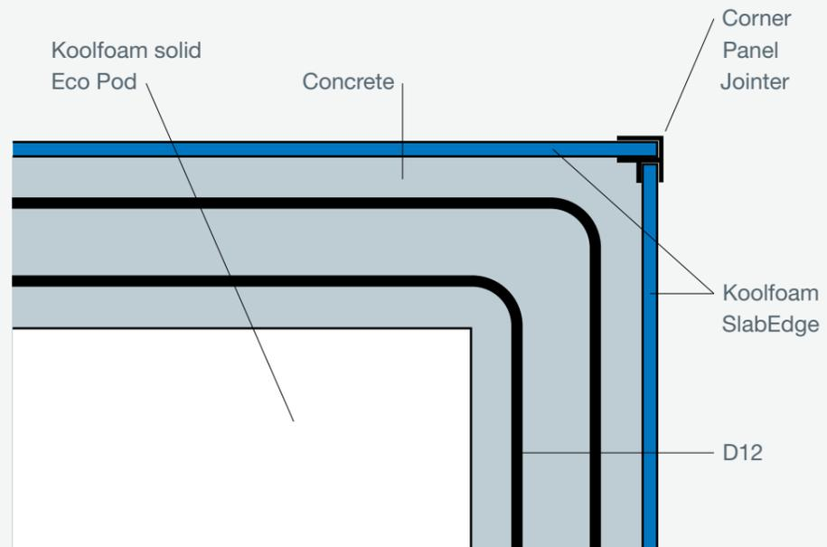
Location and placement of the KoolFoam SlabEdge system to be verified by the architect and or structural engineers. Drawings are representative examples only. Application of Koolfoam SlabEdge to be designed in accordance with H1 Energy Efficiency Acceptable Solutions H1/VM1 H1 VM2 or Verification Methods H1/AS1 H1 AS2.
