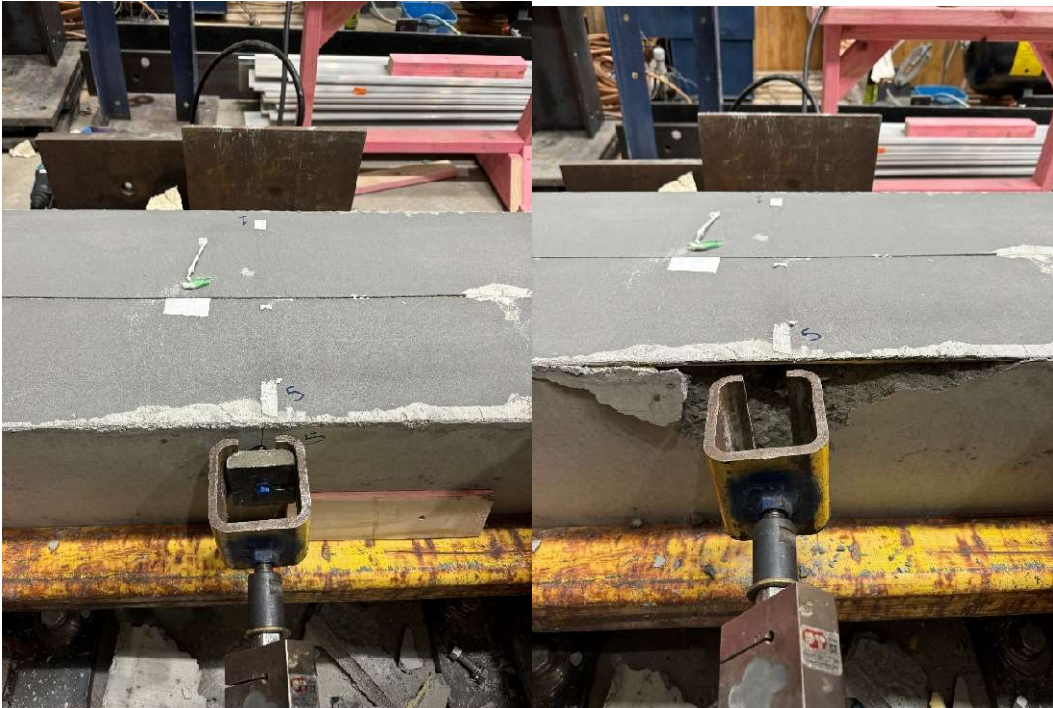
Figure 5 Failure Mode Tension (Concrete anchor)
