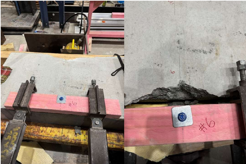
Figure 7 Failure Mode out of plane (Concrete anchor)
